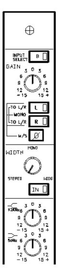
The effect return VCA master is only fitted to consoles with the optional VCA Grouping inputs. The effects return section may be controlled by the VCA masters.
